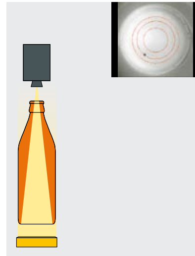
Base inspection unit
