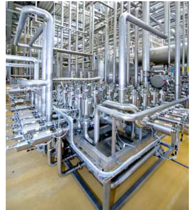
Double-seat valve manifold for central distribution of the cleaning media
